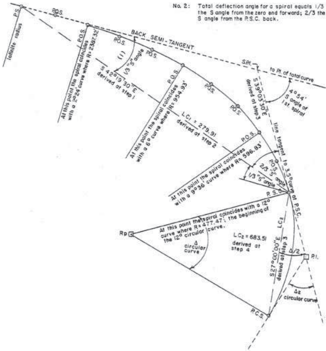
THE FRONT END OF THE THREE-SPIRAL CURVE (Exaggerated Scale)
